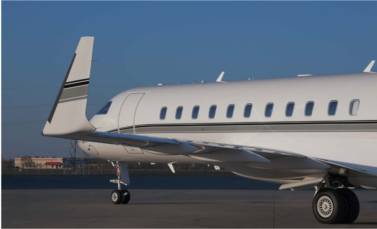
Exterior - Winglet Detail
